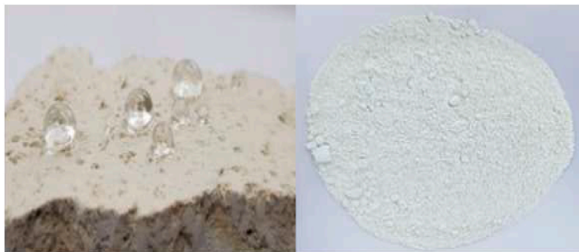
Fig. 4. Water-repellent impregnated natural zeolite [38].
